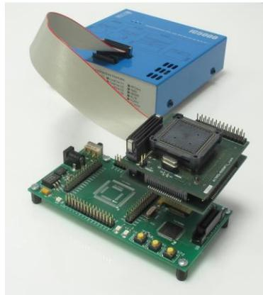
**Figure 4** Complete iSYSTEM User Trace System
