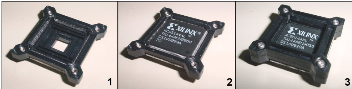
IA144YAM-SOLDER used to insert the CPU directly to the target
