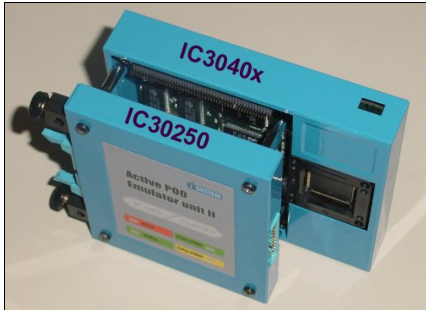
HC(S)12 ActivePOD ready for assembly
