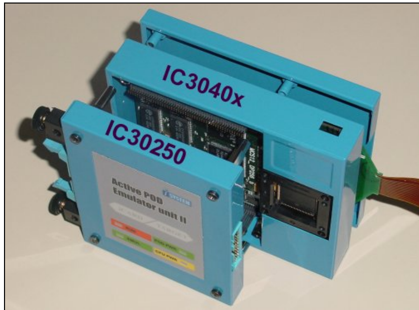
HC(S)12 ActivePOD ready for assembly
