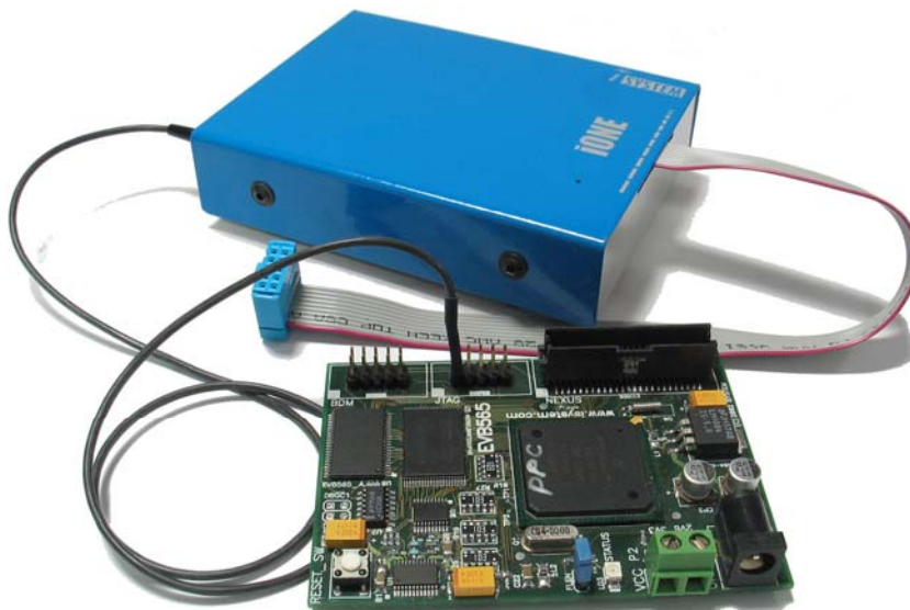
The ground wire connecting the target and iONE
