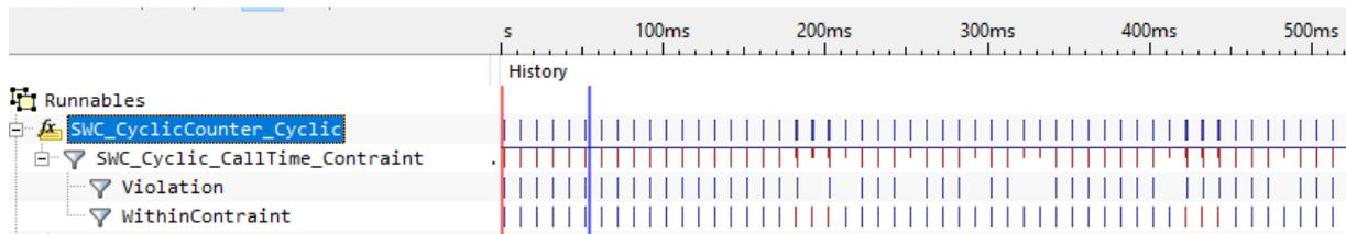
Figure 16: iSYSTEM Profiler Timeline of the Runnable “SWC\_CyclicCounter\_Cyclic” including a Profiler Inspector which checks for Violations of a specified Call Time Timing Constraint.
