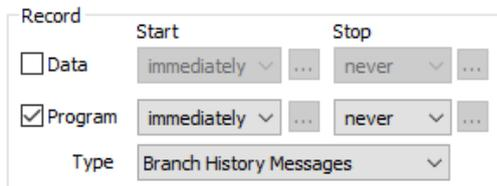
Figure 4: Program Trace enable on a PowerPC Nexus Trace Module
