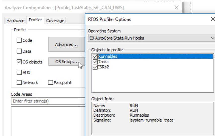
Figure 14: Profiler Configuration for Runnable Profiling based on Program Trace
