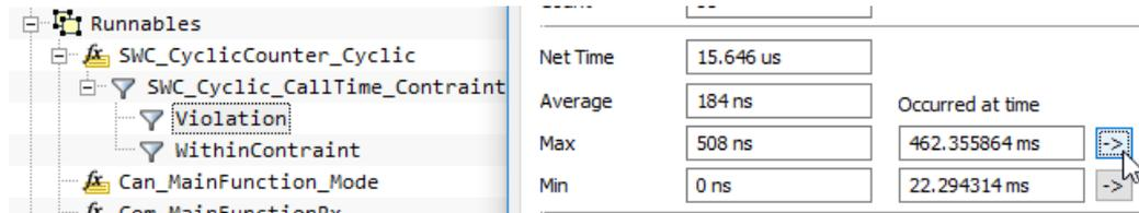
Figure 18: Net Time Properties for the “Violation” Inspector Object. The maximum Timing Violation of 508ns occurred at trace time stamp 462.35ms.
