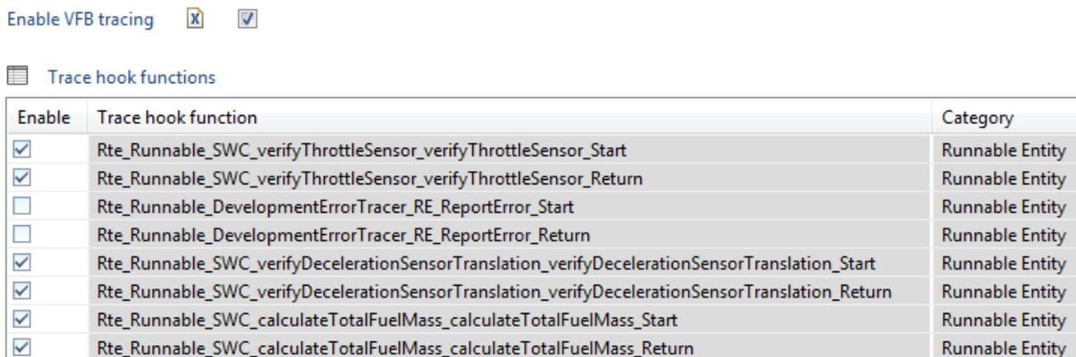
Figure 12: VFB Trace Hook Function Selection in the EB tresos RTE Editor
