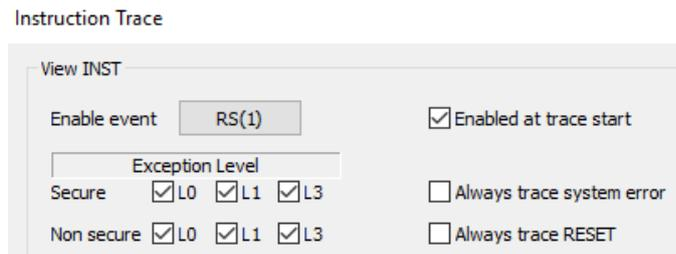
Figure 3: Program (i.e. Instruction) Trace enable on a Cortex R7 ETMv4
