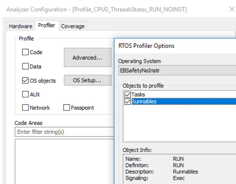
Figure 2: Profiler Configuration for Runnable Profiling based on Program Trace
