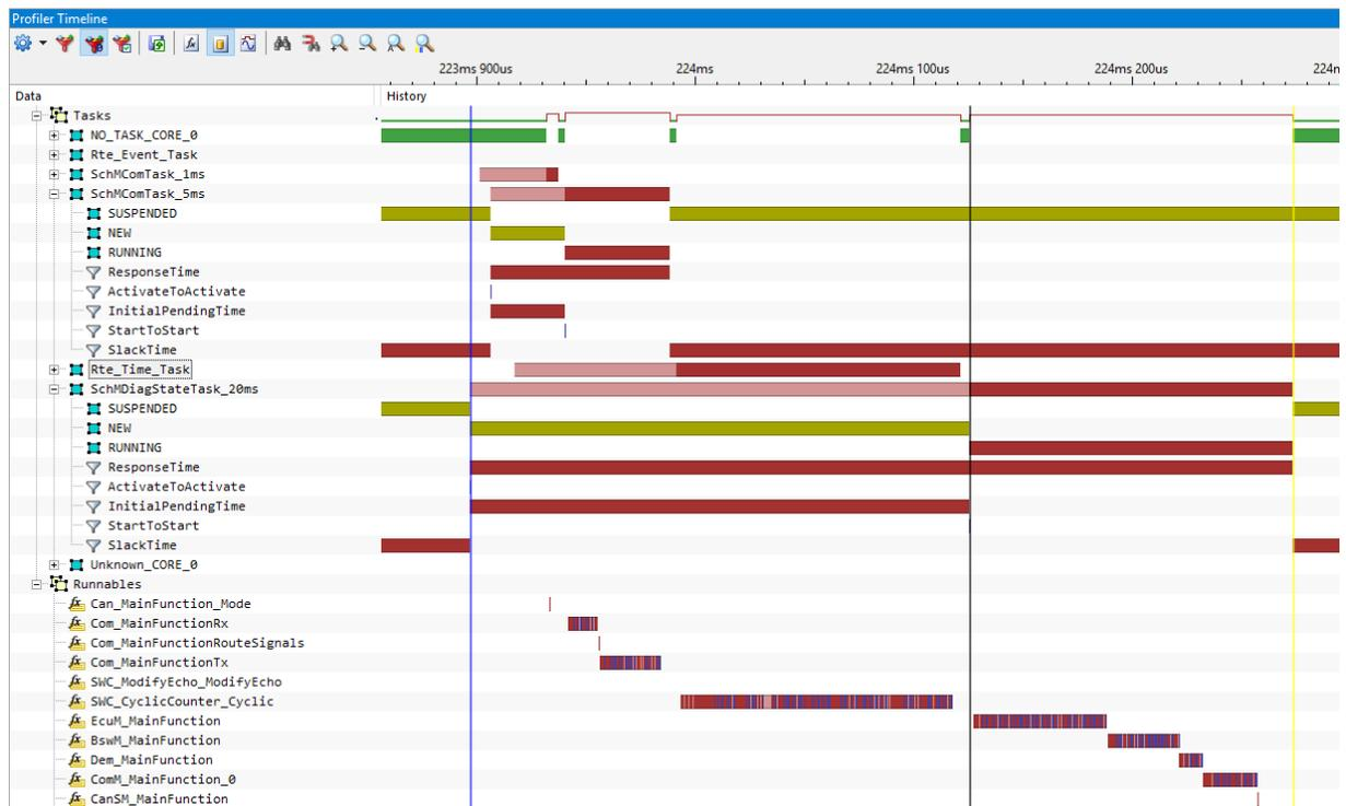
Figure 7: OS Task State and Runnable Trace in the winIDEA Profiler Timeline.
