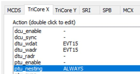
Figure 6: AURIX MCDS Compact Function Trace enable
