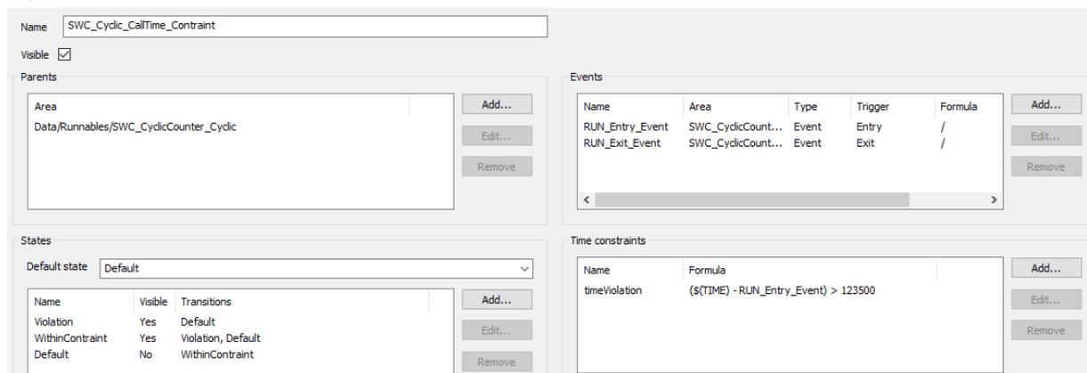
Figure 21: Configuration Dialog for the Inspector “SWC\_Cycle\_CallTime\_Constraint”
