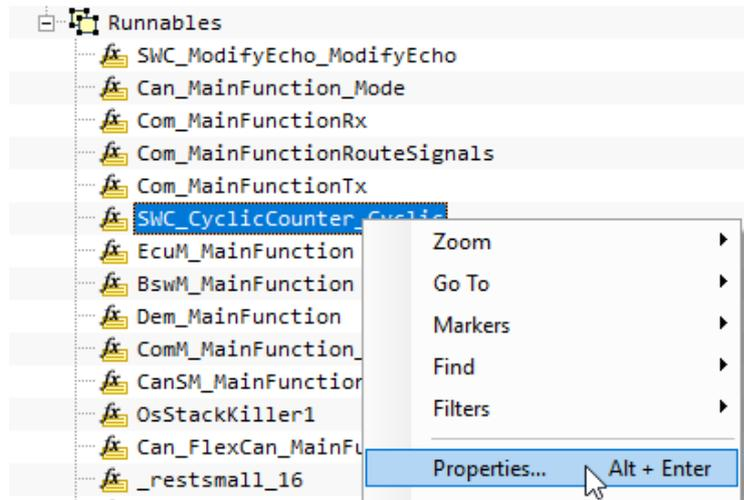
Figure 10: Opening the Properties View for a selected Profiler Object, for instance the Runnable SWC\_CyclicCounter\_Cyclic
