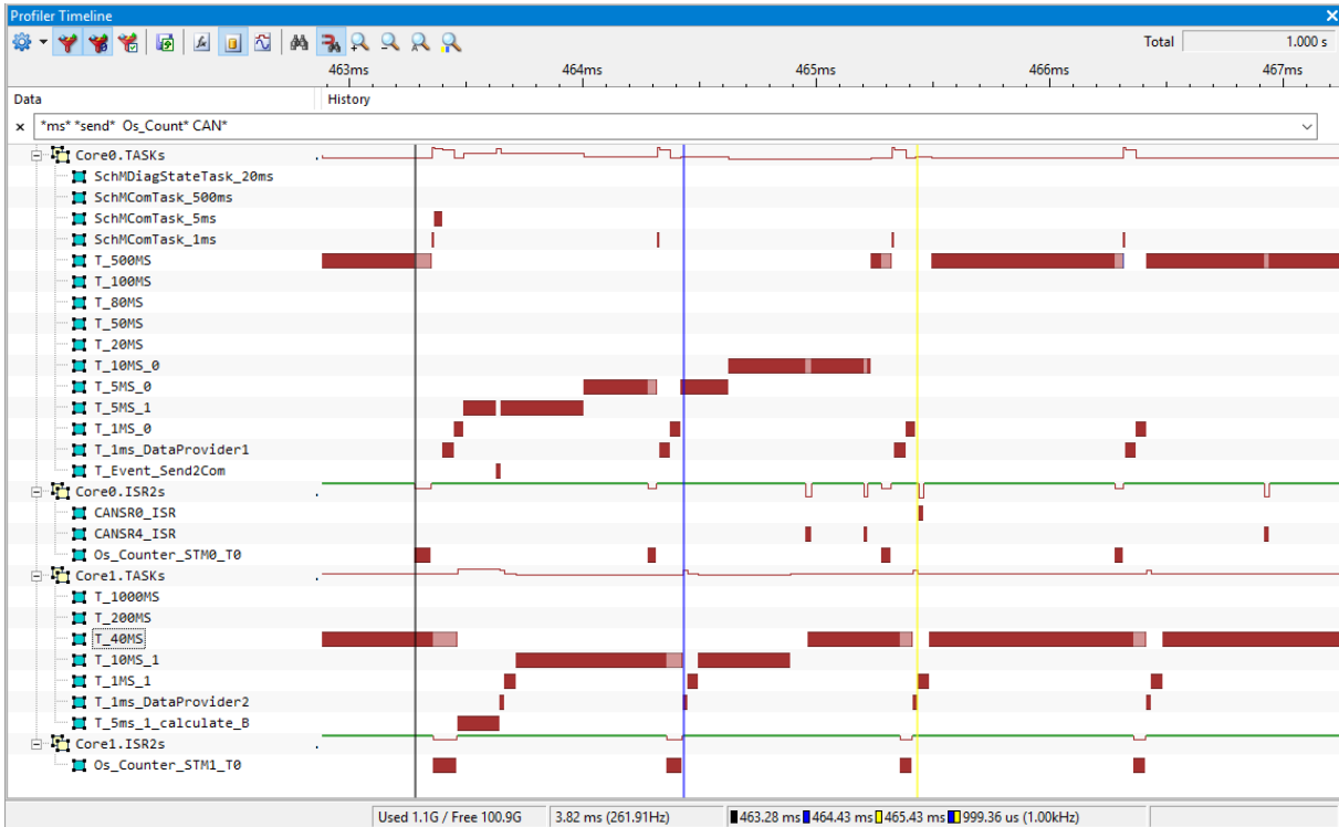
Figure 2: Running Task/ISR2 Trace in the winIDEA Profiler Timeline.
