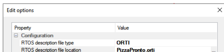
Figure 2: Operating system configuration for Running Task/ISR profiling of the application with the curious name PizzaPronto.
