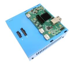
5 Tighten the IOM6 Hub with 5 screws (D) using Phillips's screwdriver.
