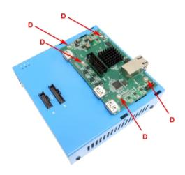
Tilt the IOM6 Hub cover and slide it over the FNet connectors.
