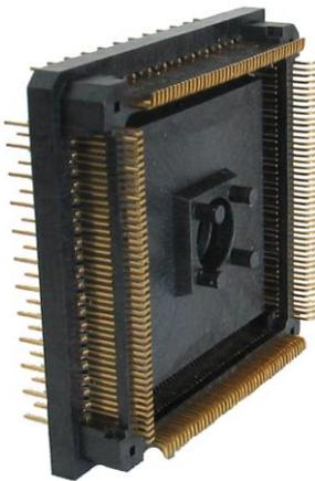
Solder part, which is being soldered to the target.
