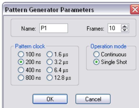
*iC2000/iC4000 Pattern Generator Parameters dialog*
